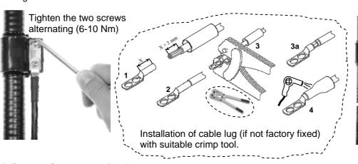
Straighten the grounding wire in the direction to the grounding point (shortest way possible). The fixation of the wire is recommended. Note the standard & local rules.
