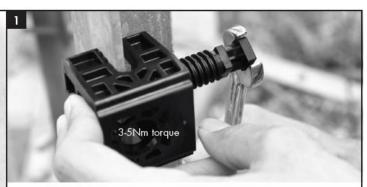
Place adapter on mounting structure. Engage  $\ensuremath{\mathcal{V}}$ " wrench on top head and tighten at a slow and steady pace. The top head is designed to snap at the correct torque. Do not tighten further.
