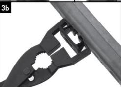
The STRT-1 tool is shown here (3b) with proper removal alignment on the base pads of the isolator.
