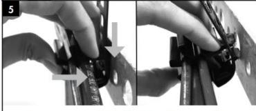
To remove: Press down with thumb and apply pressure with fingers on clip to squeeze latches together and rotate hanger out.
