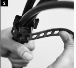
Stretch and wrap strap tightly around cable bundle expanding the corrugations until you get two strap holes to slide down onto the latches.
