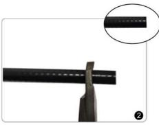
Straighten cable. Cut off the cable head.
