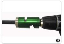
Insert the cable into the trimming tool. Select the low speed on the drill or 400~600 RPM on a variable speed drill. Trim the cable until no further debris generated.
