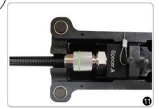
Press the trigger on the compression gun until it cycles and you hear a "pop". Do not pull or push on compression gun during compression.
