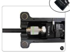
Place spacer A into the compression frame. Make sure the connector and cable both lay flat in the compression frame.
