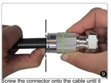
reaches the marked line. Over tighten is forbidden.
