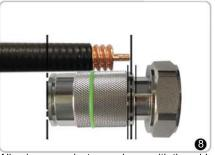
Align inner conductor as shown with the middle of two lines. Mark cable jacket in line with end of connector.
