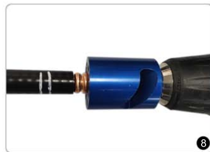
Using the low speed setting on the drill, insert exposed outer conductor into trimming tool base. Continue trimming until tool reaches cable jacket. Do not push tool beyond this point.
