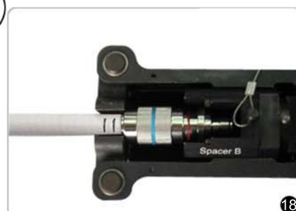
18 Make sure the connector nut is lined up against spacer B to prevent damage to the O-ring during compression.
