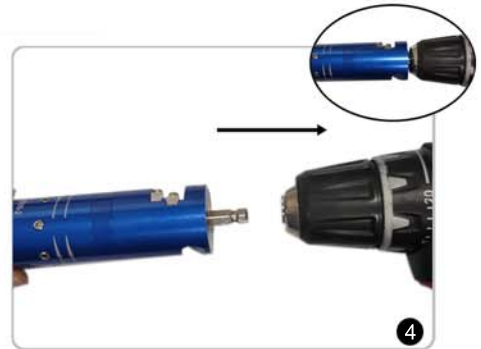
Attach the trimming tool to power drill.
