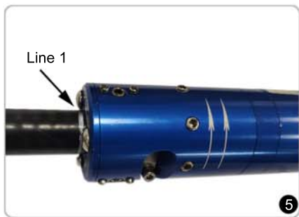
Insert the cable into the trimming tool. Select the low speed on the drill or 400~600 RPM on a variable speed drill. Trim the cable until the tool reaches line 1 on the cable.
