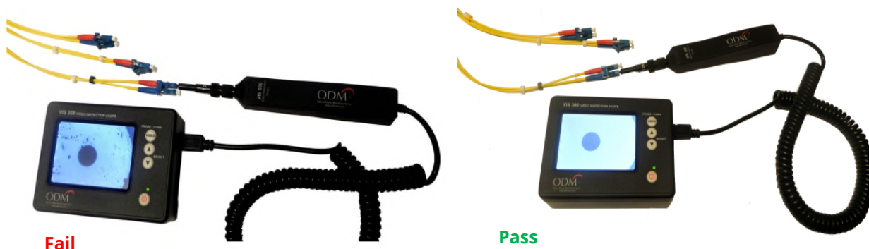
LC end-face inspection
