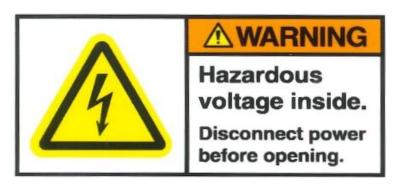
Hazardous voltages exist inside the unit. Unplug the power before servicing.
