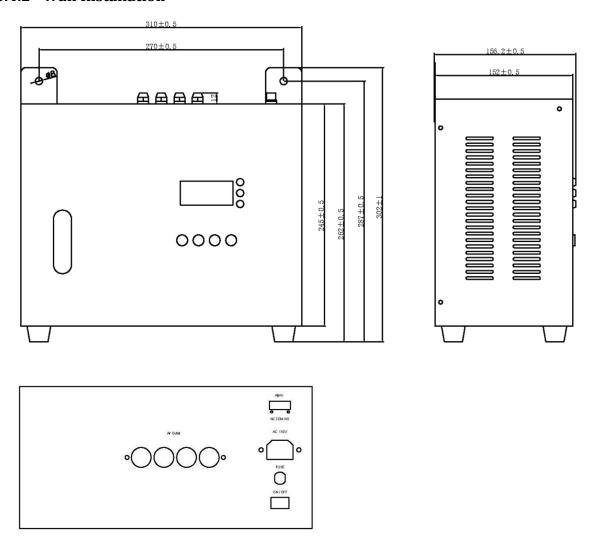
The dehydrator can be mounted on a wall using the supplied brackets. Following the hole location diagram shown in the figure.
