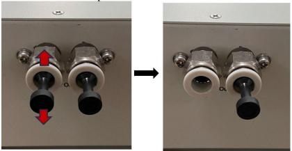
Switch on the power to activate the dehydrator and let it run for 3-5 minutes with nothing attached to the dry air outlet fitting. Check the airflow coming from the gas outlet using your finger. Disregard any alarms shown on the front panel.
