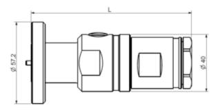
78EIA-HCA78-019 connector, dimensions in mm, L=115mm
