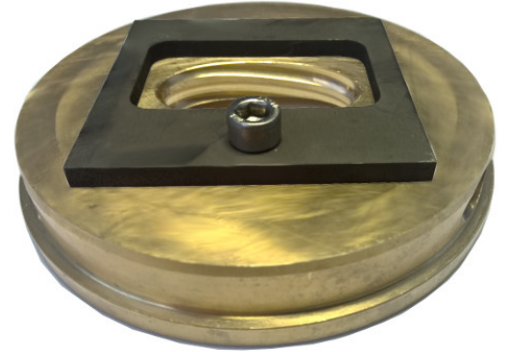
Picture shows flanging die for E65 waveguide
