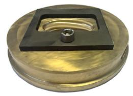
Picture shows flanging die for E65 waveguide
