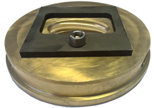
Picture shows flanging die for E65 waveguide
